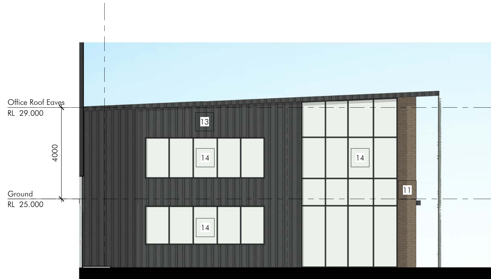
3 Office 2A - North Elevation 1 : 100
